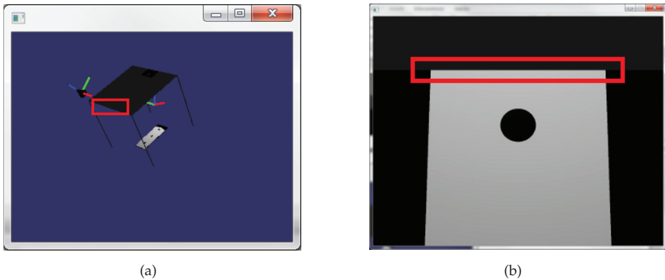
Fig. 4. (a) Preview of the whole scene (b) Camera view. The red area marks the edge of the housing that blocks parts of the object from being visible.
