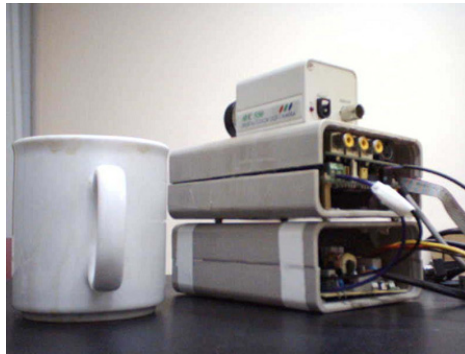
Fig. 13. FU-SmartCam : On the top, we have a low cost interlaced scan camera, in the middle we have the Vortex system, and in the bottom we have a dual output power supply. The Vortex system itself consists of two boards. The overall system is quite small.
